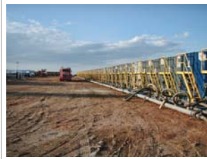
Water tanks preparing for a hydraulic fracturing job. Photo by Joshua Doubek.
